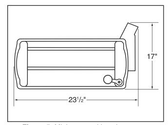
Figure 5. Minimum working clearances.
